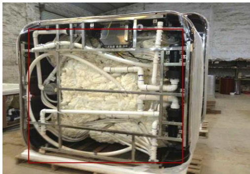
Support structure (vertical spa)
